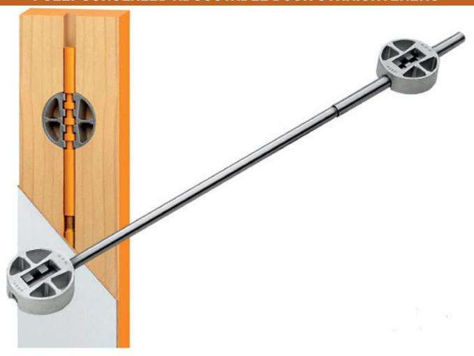
Door Adjusters are needed to avoid bending on both sliding and swinging doors. Sliding doors tend to bend in the first upper third, and hinged doors bend in the centre section. Until now these have only been available in a semi-recessed option, which brings the general appearance of your furniture down - something that all premium joinery must avoid!
